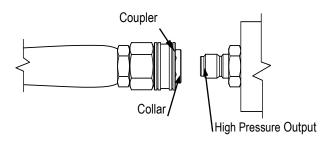
3. Release the collar, making sure it springs back and re-seats to its original (non-retracted) position. Check the connection by pulling on the hose to ensure a positive connection.
