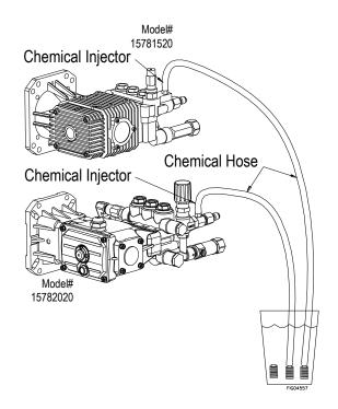
**Note:** Adding accessories (IE: telescoping wands, extra length of High pressure hose, Non factory triggers) will effect chemical injector performance or cause it not to operate at all.
